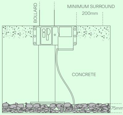
COMPACTED HARD-CORE GRAVEL (for drainage)
