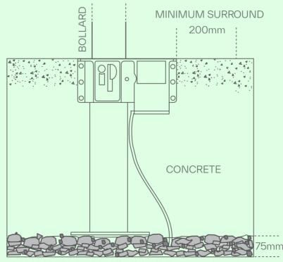
COMPACTED HARD-CORE GRAVEL (for drainage)
